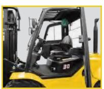
Quick easy to open hooks provide access to the engine compartment Large and spacious cab has left and right grab handles with wide openings for easy access
